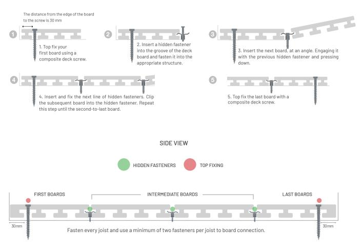
Note: Pre-drilling may be required when top fixing.
