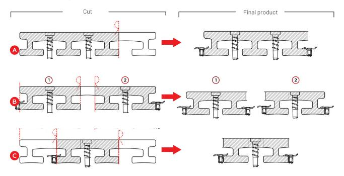
If the longitudinal profile of the ripped board is to be visible, it is good practice to install the board so that the cut face is turned inwards and the opposite face is exposed. However, in scenarios such as this, one should be able to extend the project area so that the final board can be a full board.
