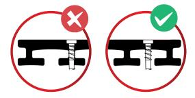
Avoid driving the top fixing screws through the web of the profile shape, this would cause cracking.
